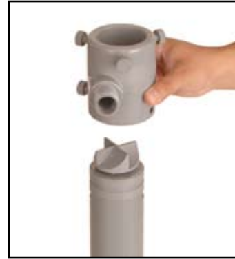
Fig. 22. Install Swiveling Impeller Housing onto Pump Body.
