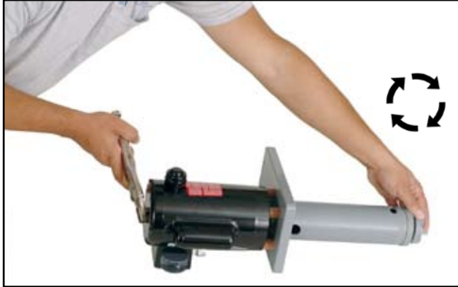
Fig. 21. Install Impeller. While firmly holding Motor Stub with vice grips, turn Impeller clockwise with hand. Impeller should spin freely and not touch pump body.
