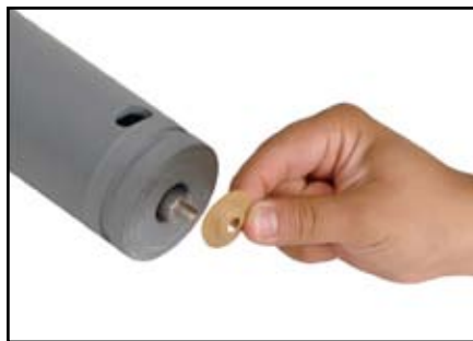
Fig. 19. Push Super Slinger over threaded end of Shaft. Note that flat side of Super Slinger must be against pump body.
