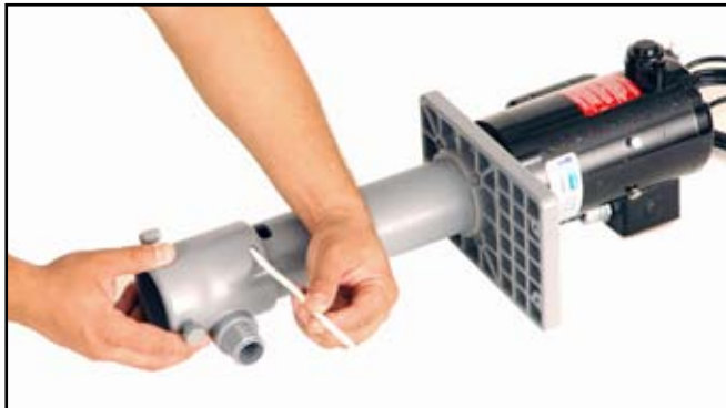
Fig. 23. Push Teflon Strap into hole while turning Swiveling Impeller Housing back-and-forth. Teflon Strap secures Swiveling Impeller Housing to Body.
