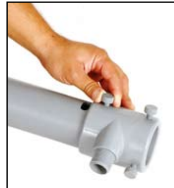
Fig. 24. Rotate Swiveling Impeller Housing to desired position for installation in tank, then tighten Lock Screw.
