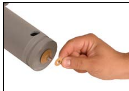
Fig. 20. Push Impeller Washer over threaded Shaft until flush against Super Slinger. Make sure Impeller Washer lays flat.
