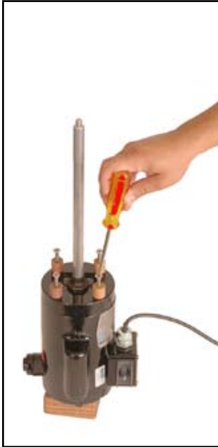
Fig. 15. After removing Fan Cover and Fan Blade from new Motor (same procedure as shown on Page 2), use Phillips-head screwdriver to remove screws from Spacers.
